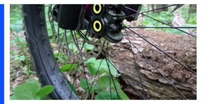
While Magura has apparently gotten varied feedback on the bite point on the lever, I found the set up using the tool-less adjustment to be just about perfect when the lever was pushed in far enough to allow one finger braking. Otherwise the brakes can be set up to facilitate two finger braking if that's your preference. As with almost every brake we've tested with a bite point adjustment, it went unused.
